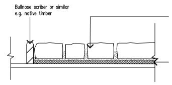
Selected 'Eldorado' stone veneer over 'Stone-Tite' mortar system to 7.5mm 'BGC Stonesheet' fixed with s/s screws and washers
