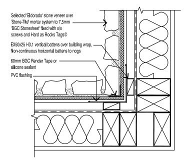
NOTE: EX50X25 BATTENS CAN BE SUBSTITUTED WITH EX50X50 WHERE APPROPRIATE
