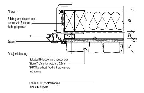
NOTE: EX50X25 BATTENS CAN BE SUBSTITUTED WITH EX50X50 WHERE APPROPRIATE
