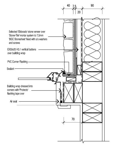
NOTE: EX50X25 BATTENS CAN BE SUBSTITUTED WITH EX50X50 WHERE APPROPRIATE
