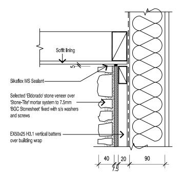
NOTE: EX50X25 BATTENS CAN BE SUBSTITUTED WITH EX50X50 WHERE APPROPRIATE
