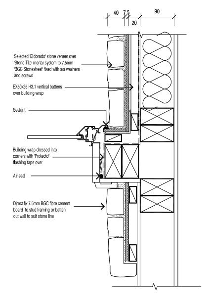
NOTE: EX50X25 BATTENS CAN BE SUBSTITUTED WITH EX50X50 WHERE APPROPRIATE
